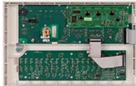
*rear view of front door with zone LED kit fitted*
