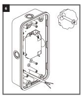
7. Terminate the supply cable into the terminal block on the rear of the gear tray, observing correct polarity. Ensure all conductors are fully sleeved and insulated against heat. This fitting is Class II Double Insulated. No earth connection is required.
