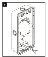
**6.** Position and fix the base to the mounting surface, using the screws provided at the four fixing positions.
