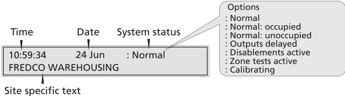
**Normal** is displayed when there are no fires, faults or pre-alarms on the system and the panel's day/night (building occupied/unoccupied) facility HAS NOT been set up by the system engineer.
