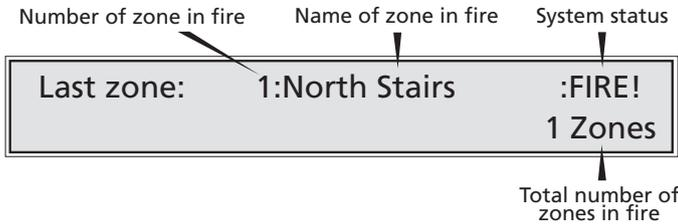
Pressing the More Information button will display the actual device that has triggered the fire condition, for example:
