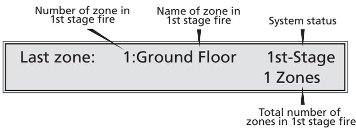
If the 1st-Stage alarm is in a zone set up with a zone dependency function:
